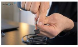
**Caution:** Connect the serial cable to the byteDEVKIT STM32MP1 as shown. The **black cable** must point towards the USB OTG connector.
